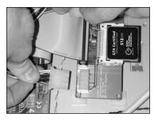
Connecting the Power Supply to the 4-pin Power Port of the IDE Adapter Board
